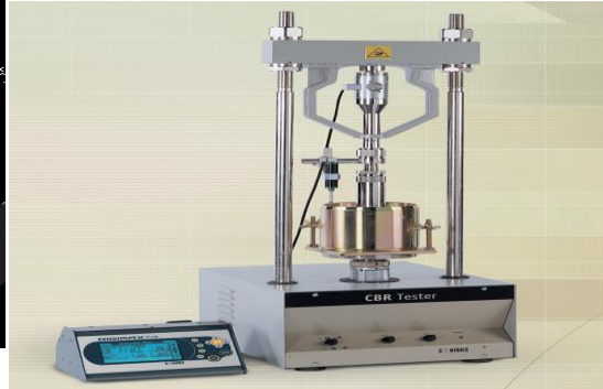
Figure 3.25: Essai CBR (California Bearing Ratio)
